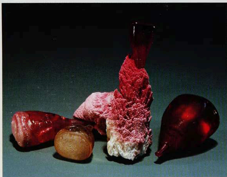
301. VERNEUIL PROCESS: Boules grown by A. Verneuil and associates ~ 1900; upright boule ½ inch.
