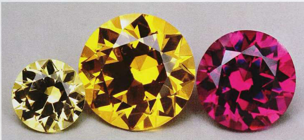
325. SYNTHETIC GARNETS: yellow = dysprosium- aluminum; orange = samarium- gallium; red = neodymium-gallium; all 1-5 carats.
